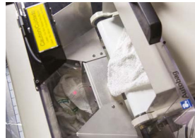
Optional Laser Level Control System Monitors the bag content and overrides the counter, cycling the bagger when the count height is reached
