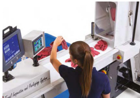
Optional Reject Count System Tracks number of pieces rejected during inspection and displays the reject count and percent of total pieces run
