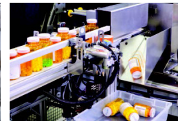
Incomplete or mismatched orders are diverted to a reject bin
