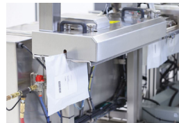
Labeled, loaded bag is automatically sealed as it exits the bagger
