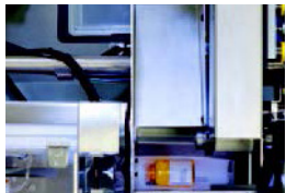
A wide bag opening enables automatic loading of single or multiple piece orders
