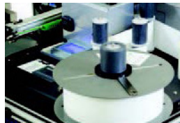
Shipping label is automatically printed and applied to bag
