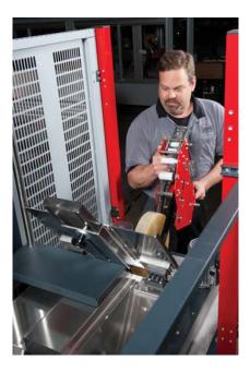
The CE-10's hinged case hold down plate allows for easy tape-head removal. The case erector's open design eliminates overhead cross members providing easy access for planned maintenance.
