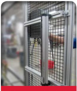
A light curtain senses the height of the incoming case, communicates with the servo and the height of the top taping head is automatically adjusted.
