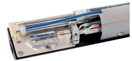
Sealtronic nozzle during start up with open gutter.
