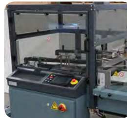
New Guarding featuring Dual Monitored Safety Circuit
